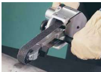
Model 11475 is ideal for grinding circumferential welds.
