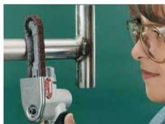
Clean and finish using non-woven nylon belts.
